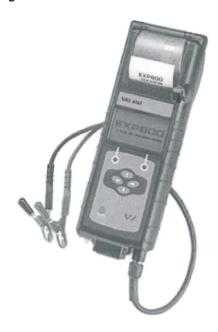
The new battery tester VAS 6161 is the successor unit for the VAS 5097A testers previously used. The new VAS 6161 is no longer a tester that checks the battery discharge under load. Instead, a measuring principle of dynamic conductance detection is employed.
