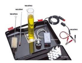
The test set can be used to identify the diesel of the affected vehicle.
