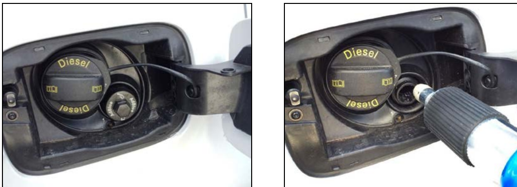
Fig.: 27 Tank inlet and nozzle
