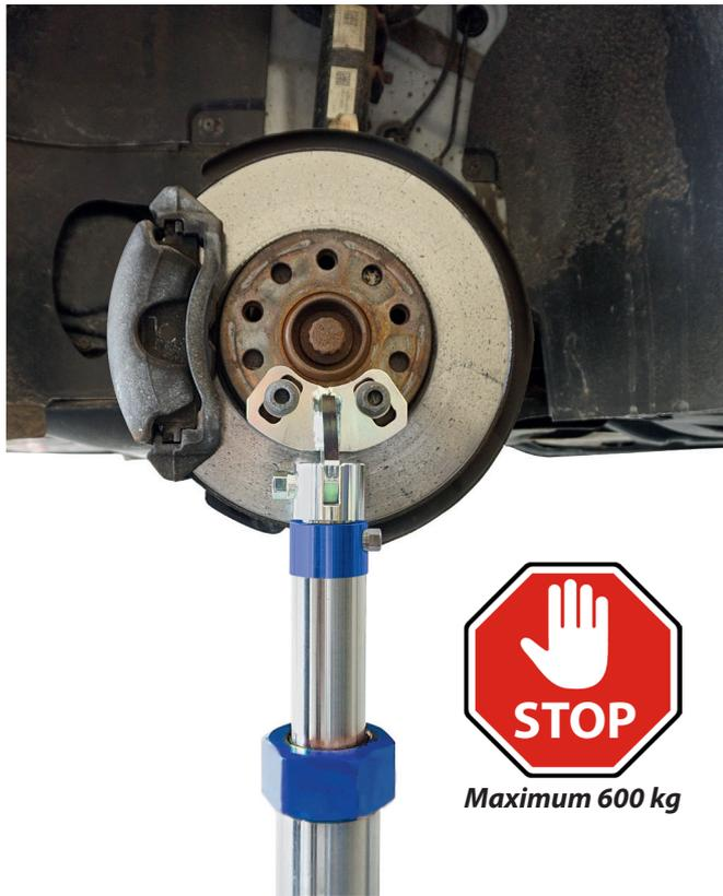
**Fig. 6:** Relieve the support device and remove it from the wheel hub.
