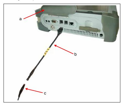
Fig. 5-5 Connecting the VAS 6558A to VAS 5051B
