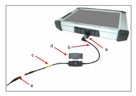
Fig. 5-4 Connecting the VAS 6558A to VAS 5052A
