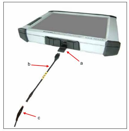
Fig. 5-3 Connecting the VAS 6558A to VAS 5052A
