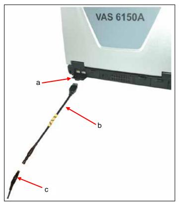
Fig. 5-6 Connecting the VAS 6558A to VAS 6150A (specified laptop)
