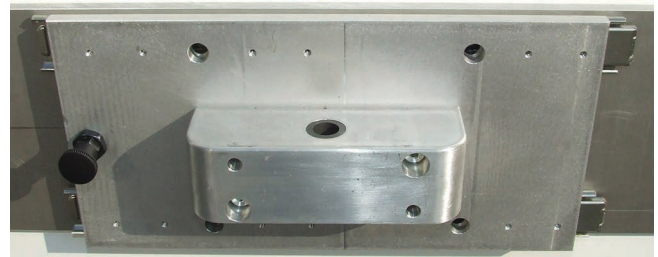
Fig. 15: Rear view of calibration board with slide unit
