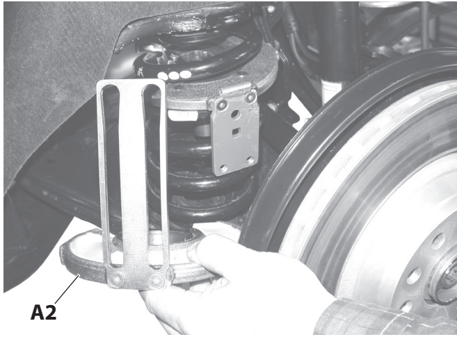
Fig. 33: Removing the pressure plate with swivel bearing "A2".
