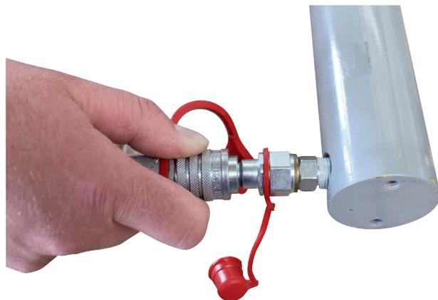
**Hydraulic hose is fully connected.**
