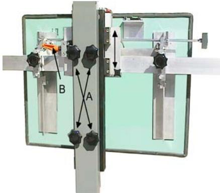
In order to preadjust the height of the calibration bar, place the complete unit “vertical sledge with calibration bar” in the desired position by means of 4 fastening nuts. (A)
