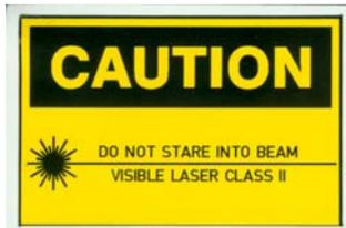
The released laser radiation corresponds to the laser class 2 (<1mW) according to EN 60 825-1. In conformity with the accident prevention regulation VBF 93, in case of casual and short look into the ray, the eyes are protected by the reflex of the eyelid shutting. Therefore you can use the laserpointer with no further safety measure. The product corresponds to 21 cfr 1040.10 (USA).
