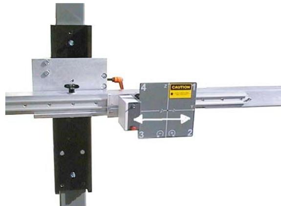
Before adjusting the calibration bar in regards to height, take off the sensors of the wheel alignment system from the ADR-calibration device.
