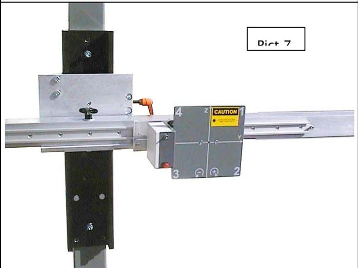
Introduce the laser box (under tensioning of the spring pressure part) with both slides into the guide beam.
