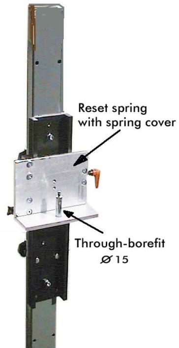
Put the through-borefit of the calibration bar onto the pin of the back plate and fasten it by means of the fastening nut.
