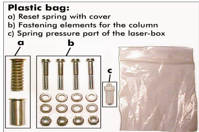
sledge (Pos.2+3) on the centre of the support by means of the fastening elements b) in the enclosed plastic bag. (Picture 2)
