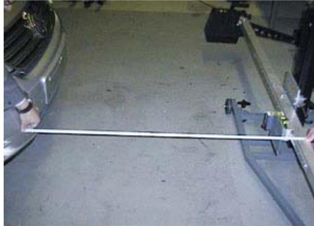
2. Place the spirit levels of the laser-box in central position by means of the three levelling screws of the calibration device.
