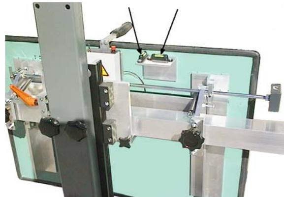
4. Slide the “Rough” calibration mirror over the Radar sensor, and fasten it by means of the springs and elastic fasteners.
