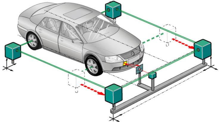
5. Turn on the device. Calibration can be called by clicking the menu "Measurement routine", sub-menu "ADR sensor calibration" or the screen button "ADR sensor calibration" (only for vehicles with ADR/ACC-equipment).
