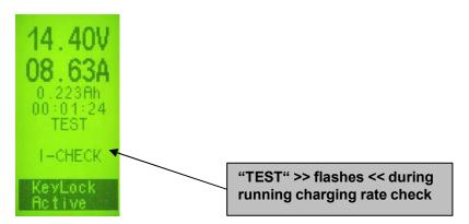
An interrupt of a running "I-CHECK" charging rate check is only possible by disconnecting the cable clamps from the battery, because of the activated "KeyLock".
