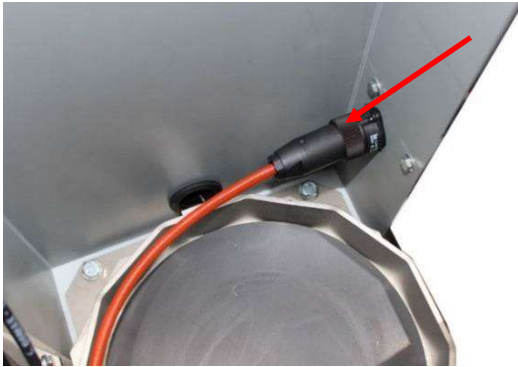
Fig. 4-33 Connecting heating band
