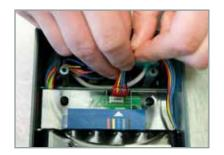
4. When you are sure that you have connected the lithium-ion battery in accordance with the instructions, screw the rear cover of the VAS 5581 back on. Your HV diagnosis box is now ready for use.
