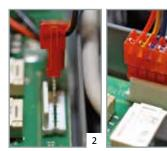
Attaching the plug in a manner contrary to the instructions specified above may cause defects, or result in a short-circuit, as soon as the VAS 5581 is switched on.
