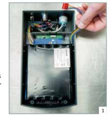
3. Attach the plug to the circuit board of the device so that the white socket guide rail on the circuit board is able to engage the recess in the red battery plug as intended (refer to Figure 2 + 3).
