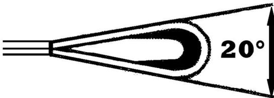
Keep the sling's seams away from the hook area and away from other lifting devices. Avoid damaging the label. If more than one product is used to lift the load, all the products must be made of the same material (to ensure the same elongation values, for example).
