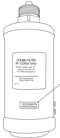
Fig. 18: Location of PIN number on filter
