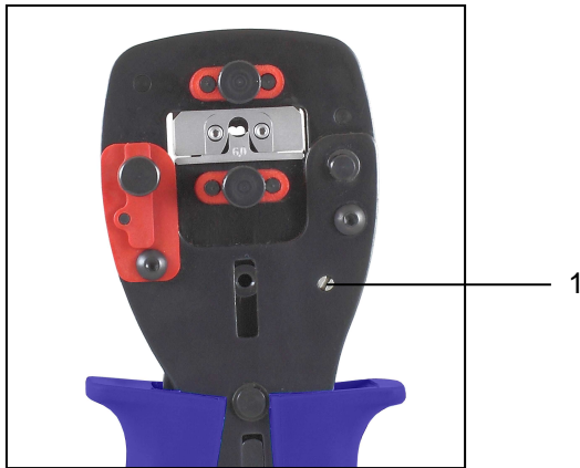
Fig. 22: Release unlocking screw
