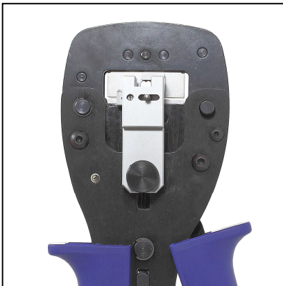
Fig. 17: Back of tool with assembled positioner
