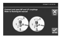
Connect and open HP and LP couplings, refer to flushing-kit manual
