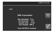
A summary of the amount of gas recovered, oil recovered, minutes of the vacuum phase and the amount of gas charged is displayed. Press for printing
