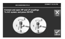
Connect and open the coupling connected to the A/C system.
