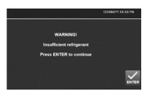
Use Tank filling procedure to increase chargeable gas to a Minimum of 3 KG
