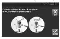
Connect and open the coupling connected to the A/C system, then press ENTER to start the vacuum phase,
