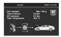
Disconnect HP coupling. Start A/C system with LP coupling connected.
