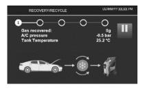
During the recovery phase, the machine displays the quantity of refrigerant recovered.
