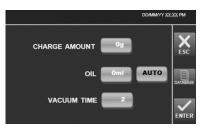
Select the OIL display zone, then use the keys 0 to 9 to type the volume of oil to be injected, or select AUTO to reintegrate the same quantity of oil extracted during Recovery.
